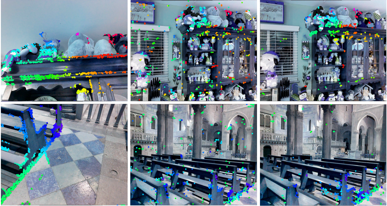
Figure 6. The scale invariance. The left, middle and right column are the nearest neighboring correspondences using feature representation from the GoogLeNet pretrained on ImageNet, the model learned without spatial transformer, and the model learned with spatial transformer respectively
